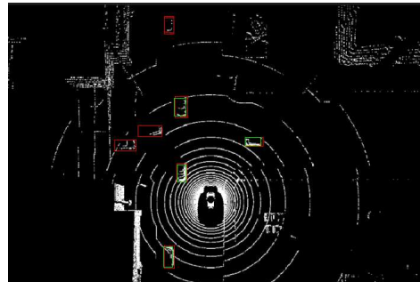
(f) Detections vs Ground Truth in PCSim Velodyne HDL-32, with Real2Sim
