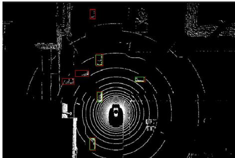
(e) Detections vs Ground Truth in PCSim Velodyne HDL-32, without DA
