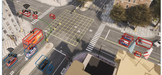
Fig. 1: Illustration of CP to accurately predict the movement of surrounding agents. Red bounding boxes are detected by CAV 1 and blue bounding boxes are only detected by CAV 2. The predicted trajectory of an agent is shown in green.
