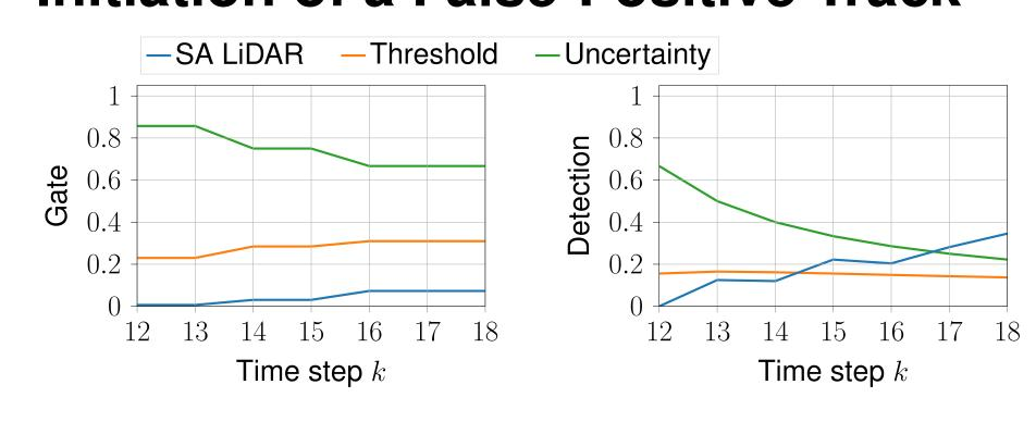
SA measures of a false-positive initiated track in Sequence 10 of the KITTI tracking dataset [2]. The false-positive track can be identified by the SA module. Firstly, the detection opinion exceeds the threshold before the deletion algorithm catches the track. Secondly, the uncertainty of the gate opinion remains high due to missed detection.
