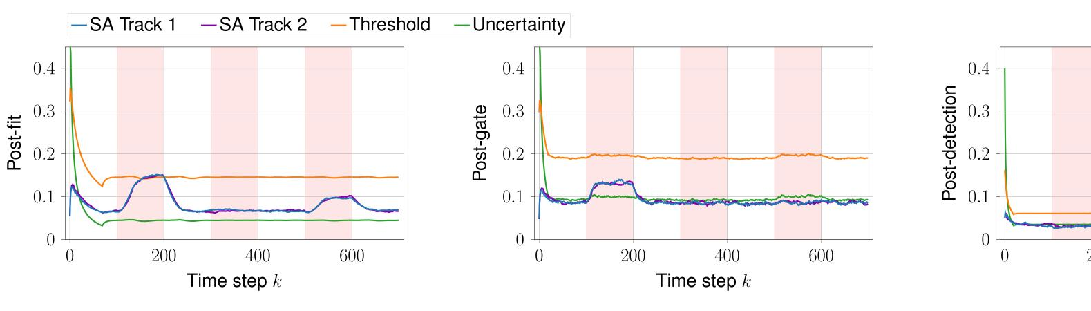
The full SA Post module results are shown to monitor the overall tracking performance. Because the Sensor 1 disturbances influence both tracks, both SA measures increase, leading to small violation reports in the post-fit and post-detection opinions.
