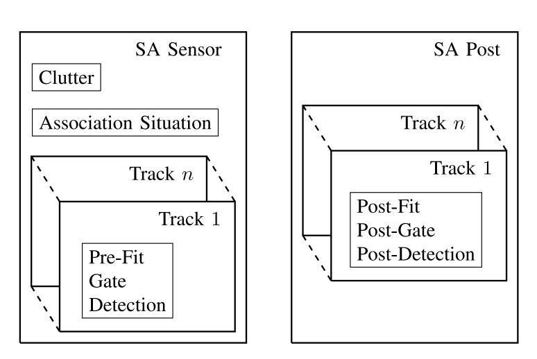
Overview of the implemented self-assessment (SA) module for multi-object tracking (MOT). The SA Sensor assesses each sensor's specific assumptions, and the SA Post assesses the algorithm's overall assumption fulfillment for each track.
