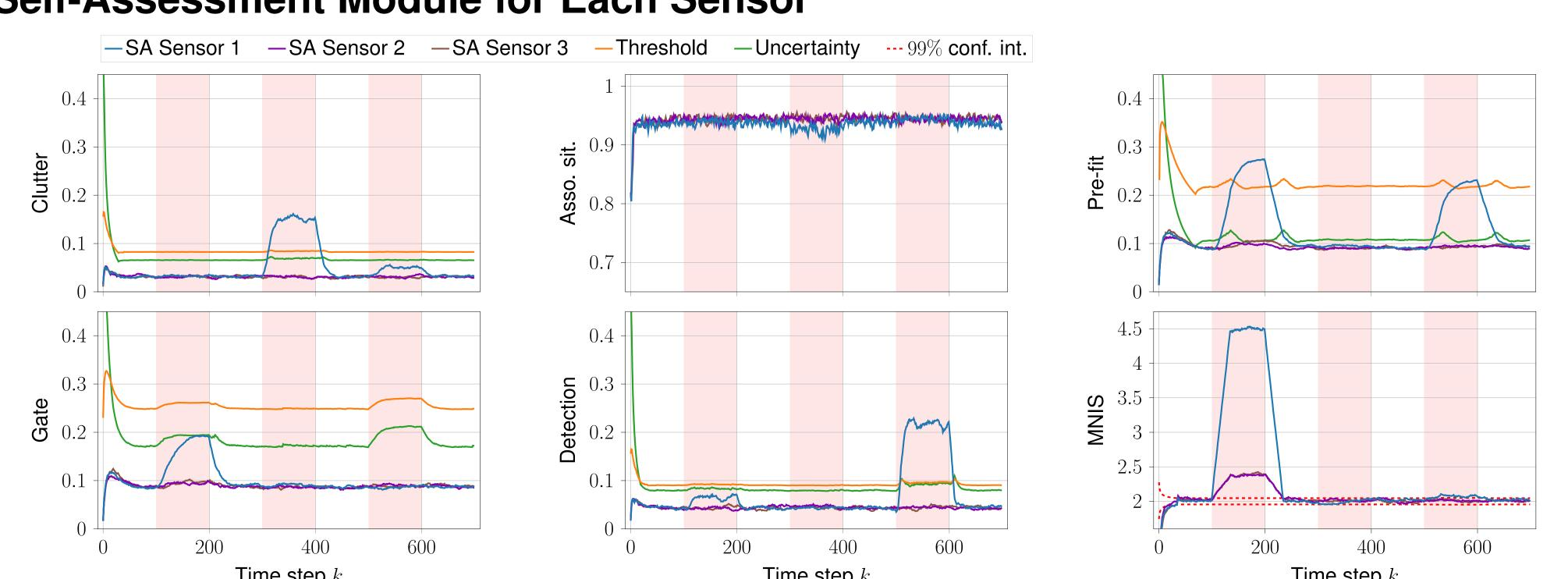
The full SA Sensor module results for all three sensors are shown and compared to the time-averaged multi-target normalized innovation square (MNIS) [1]. Sensor 1 is disturbed in its measurement noise, clutter rate, and detection probability assumptions, whereas Sensors 2 and 3 work properly. Red shadows indicate these disturbances, which are monitored by the SA module. A violation is reported when the SA measures exceed the thresholds or the confidence interval (conf. int.).
